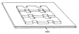
Figure 2 Schematic of a Planar Tugboat Traveling-Wave Structure (3 cells illustrated)
