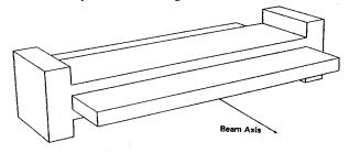
Figure 1 Schematic of a Planar Barbell Cavity
