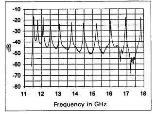
Figure 4 TM Modes frequency Spectrum of a Barbell Cavity as Measured with a HP8510C Network Analyzer
