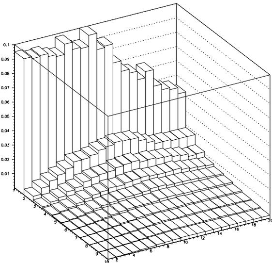
Figure 1: Energy deposition in Cu target with 28 tesla solenoid magnetic field.
