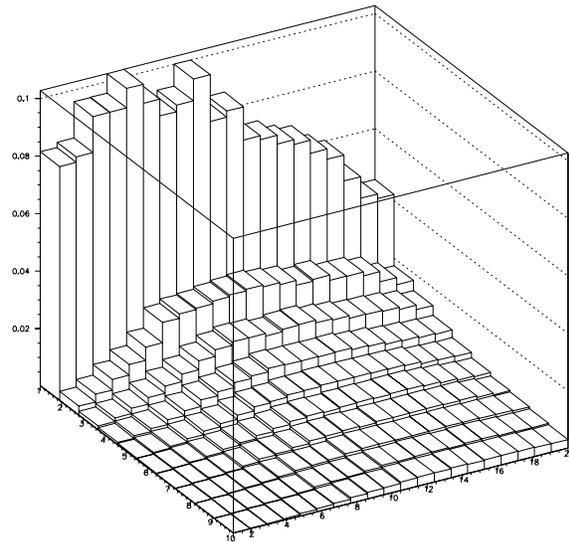
Figure 2: Energy deposition in Cu target without magnetic field.
