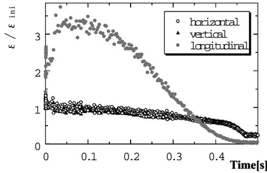
Figure 6: Time evolution of rms emittances of a laser-cooled  $^{24}\text{Mg}^+$ -beam under the influence of a coupling cavity. The longitudinal tune has been set at 0.04 while the two transverse tunes are roughly equal to 3.1. Note that an ordinary rf cavity is sitting at a dispersive position. We thus have synchrotron coupling not only by a coupling cavity but also by dispersion at the ordinary cavity.
