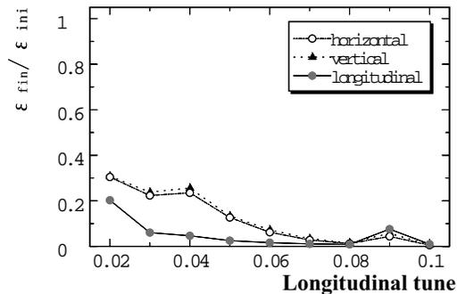
Figure 7: The rms-emittance ratio  $\varepsilon_{fin}/\varepsilon_{ini}$  vs. longitudinal tune in the coupling-cavity scheme.
