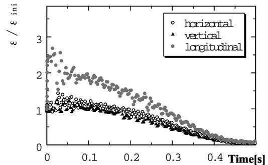
Figure 1: Time evolution of root-mean-squared(rms) emittances of a laser-cooled  $^{24}\text{Mg}^+$ -beam.  $\varepsilon_{ini}$  denotes the initial value of the rms emittance. An ordinary rf cavity has been set 10 meters away from the cooling section where the size of dispersion is 2.15 meters.
