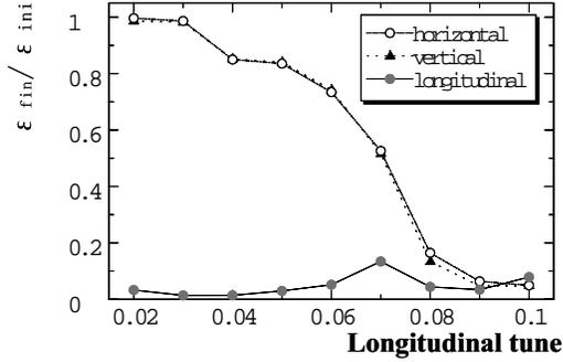
Figure 2: The rms-emittance ratio  $\varepsilon_{fin}/\varepsilon_{ini}$  vs. longitudinal tune in the dispersive coupling scheme.  $\varepsilon_{fin}$  stands for rms emittance after laser scan is completed.
