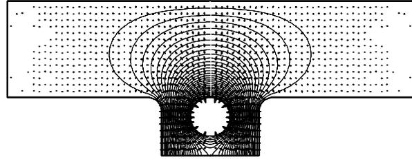
Figure 4: The approximate electric field and equipotential line of the coupling cavity. Only the lower half of Fig.3 has been shown.
