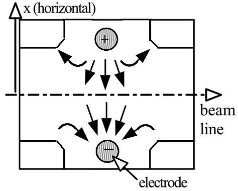
Figure 3: A possible geometry of coupling cavity.
