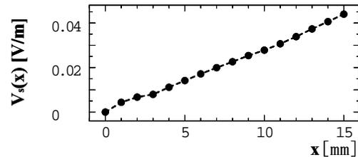
Figure 5: The dependence of the effective longitudinal electric field strength on the transverse coordinate. The absolute value of the electrode voltage has been set at 1 volt.
