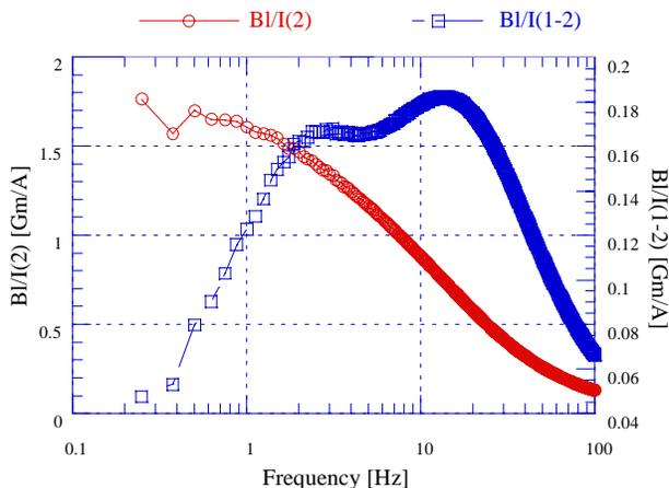
Figure 1: Magnitudes of the vertical field strength per current  $B \ell(\omega)/I(\omega)$ .  $B \ell / I(2)$  for magnet BH2 and  $B \ell / I(1-2)$  for the difference between magnets BH1 and BH2.
