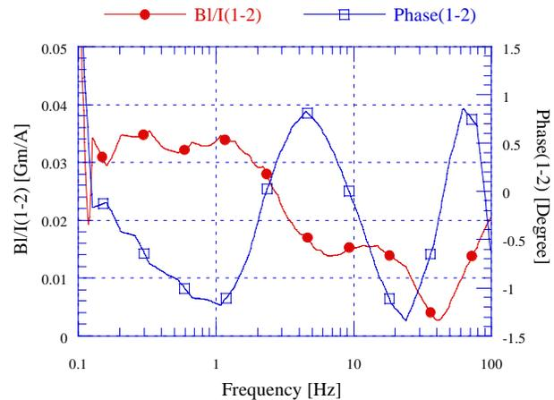
Figure 4: The differences of the magnitude,  $B \ell / I(1-2)$ , and phase delay, Phase(1-2), of the AC responses between magnets BH1 and BH2 with the three methods of flux compensation.
