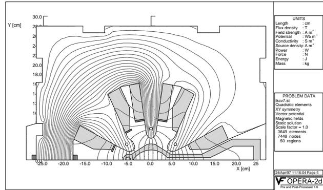
Figure 3: Upper half of the 2-D cross section of the magnet laminations, magnet coils, and vacuum chamber along with flux lines for DC current. The flux-damping coil and copper sheets for the flux shielding on two magnet poles are shown
