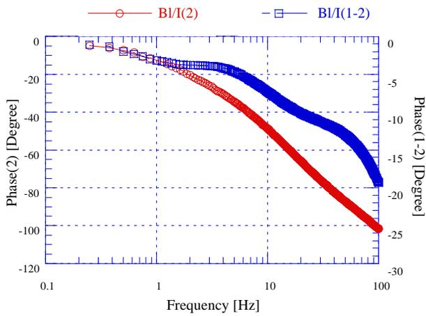
Figure 2: Phase delays of the vertical field strength per current  $B \ell (\omega)/I(\omega)$ . Phase(2) for magnet BH2 and Phase(1-2) for the difference between magnets BH1 and BH2.
