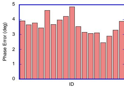
Figure: 3 Rms phase errors of all the APS 33 mm undulators, at a gap of 11.5 mm.
