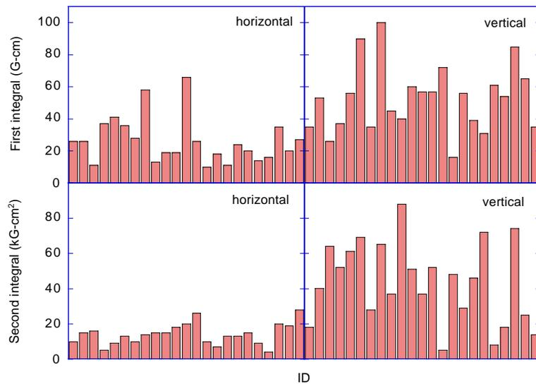
Figure: 1 First and second integrals of the vertical and horizontal components of the magnetic field through each of the IDs, as measured in the APS magnetic measurement facility.
