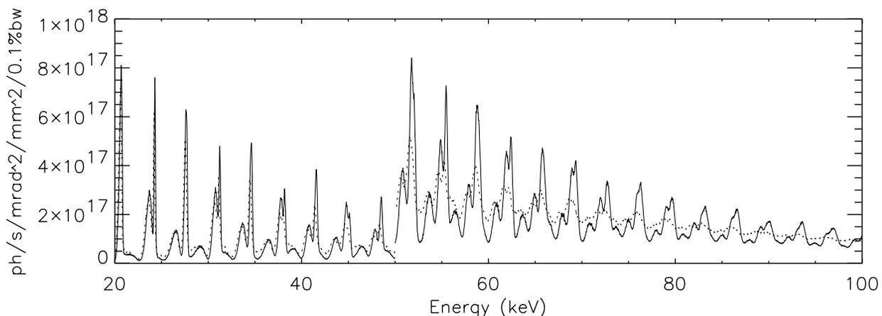
Figure: 4 Calculated on-axis brilliance, beginning at the 6th harmonic. The solid line is for the 33-mm-period undulator with the smallest rms phase error (2.5 degrees), and the dotted line is for an undulator with an rms phase error of 4.6 degrees, at 11.5 mm gap. *The brilliance above 50 keV has been multiplied by a factor of 4 for clarity.* While this difference in rms phase error has no effect at lower energies, it would affect the brilliance at higher energy.
