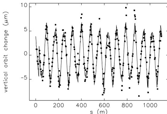
Figure: 2 Difference in vertical orbit for two different ID gaps, as a function of position around the ring. The points are the measured displacement values, and the line is the fit from the simulation. The ID is located at about 25 m.
