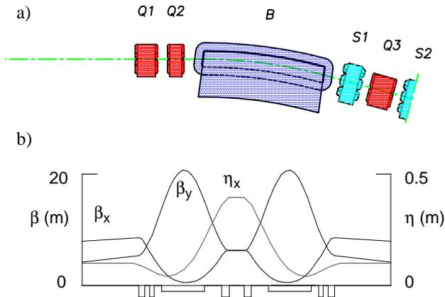
Figure 1 a) Physical layout of one half cell. b) Machine functions for one full cell.
