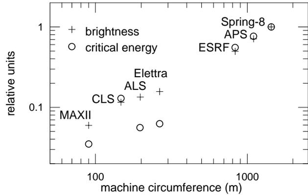
Figure 2: Relative brightness and critical energy vs machine circumference.
