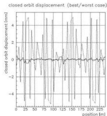
Figure 5: Closed orbit distortion for best/worst sorting
