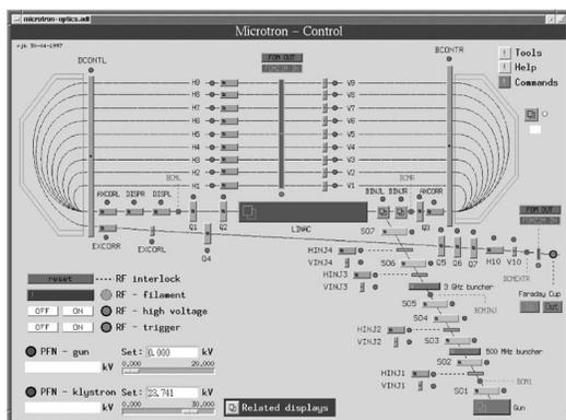
Figure 7: EPICS control panel of the race track microtron
