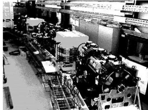
Figure 4: The first assembled achromat with multipole lenses preadjusted on 3 girders and the two dipole magnets inbetween located on individual stands.
