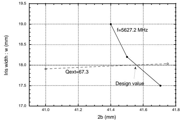
Figure 7: Determination of coupler dimensions
