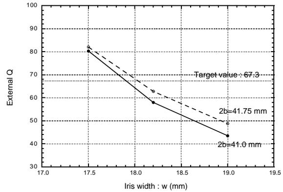
Figure 6: External Q of coupler cell.
