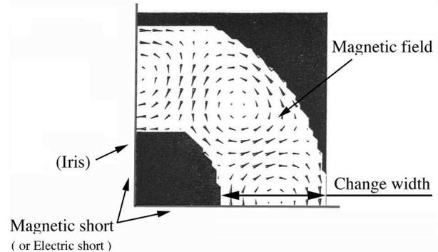
Figure 3: Geometry used in waveguide calculation by MAFIA. The arrows indicate the magnetic field under magnetic boundary condition.
