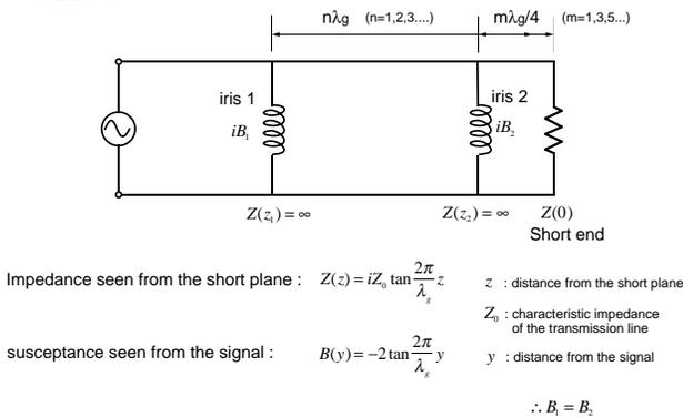
Figure 2: Simplified equivalent circuit model of two-iris coupler.
