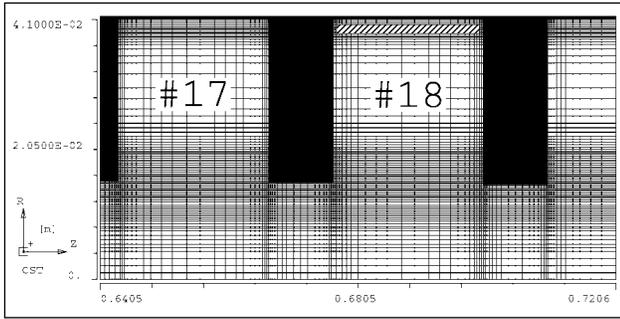
Figure 1: Three cells out of the 36-cell structure. Cell #18 with the damping material (hatched).
