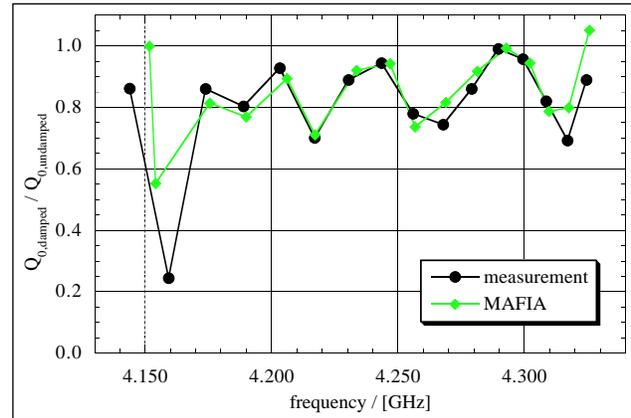
Figure 2: Comparison of calculated and measured damping effect (reduction of  $Q_0$ ).
