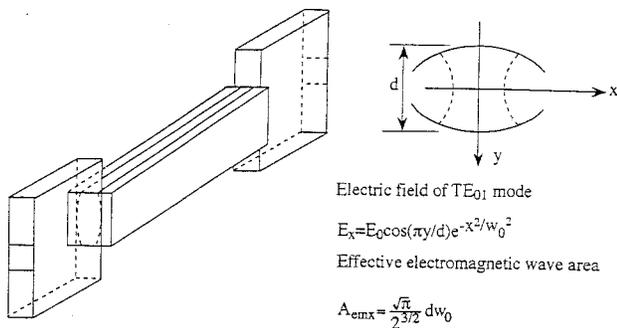
Fig. 1. The resonator.
