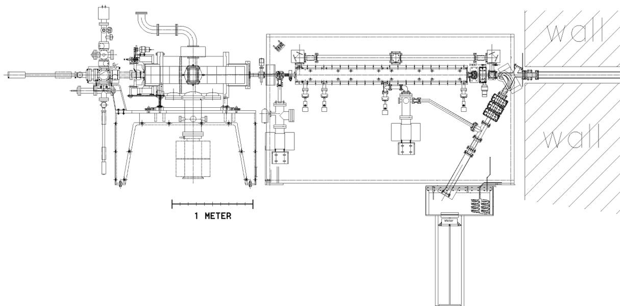
Figure 1. Experimental setup of the regenerative amplifier FEL.
