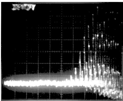
Figure 5. Fast buildup of RAFEL to saturation.
