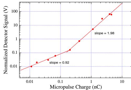
Figure 3. Plot of attenuation-corrected HgCdTe signal vs. micropulse charge on log-log scale.
