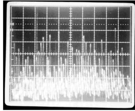
Figure 2. Oscilloscope trace of SASE at 16  $\mu\text{m}$  as detected with a helium cooled Cu:Ge detector.
