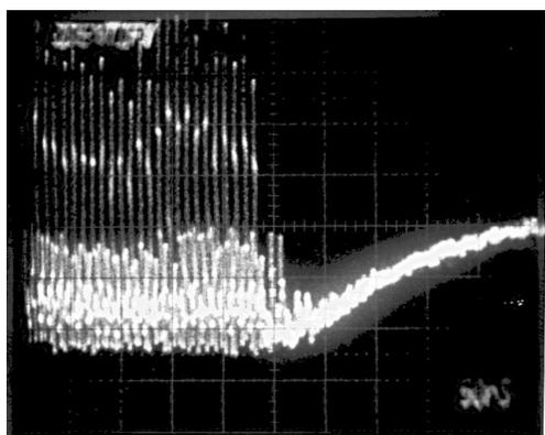
Figure 6. RAFEL ringdown shows optical power decaying by a factor of 3 in successive passes.
