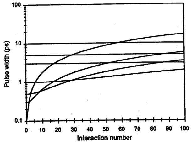
Figure 2 Plot of pulse duration vs. number of interactions for various starting values of pulse lengths.
