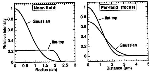
Figure 1 Near- and far-field spatial profile of equal-energy beams which pass through a 5-cm diameter aperture with minimal diffraction and the focused profile of each beam.
