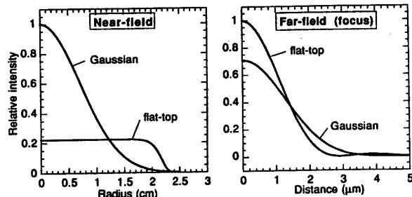
Figure 1 Near- and far-field spatial profile of equal-energy beams which pass through a 5-cm diameter aperture with minimal diffraction and the focused profile of each beam.
