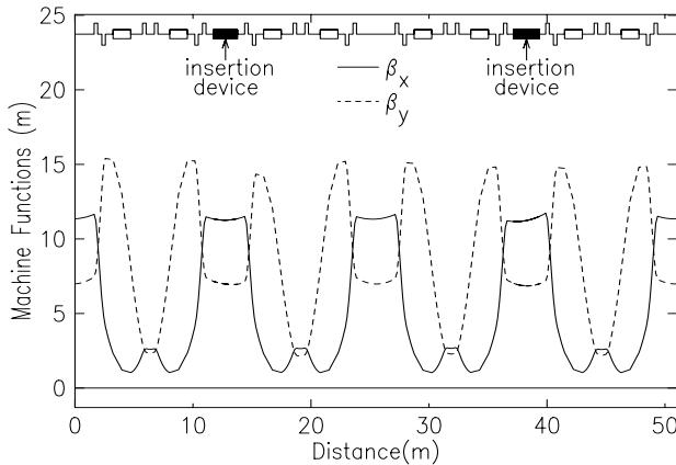
Figure 2: The  $\beta$ -functions in the NSLS VUV Ring calculated by LOCO as described in Section 2, after the periodicity restoration described in Section 3 was applied.
