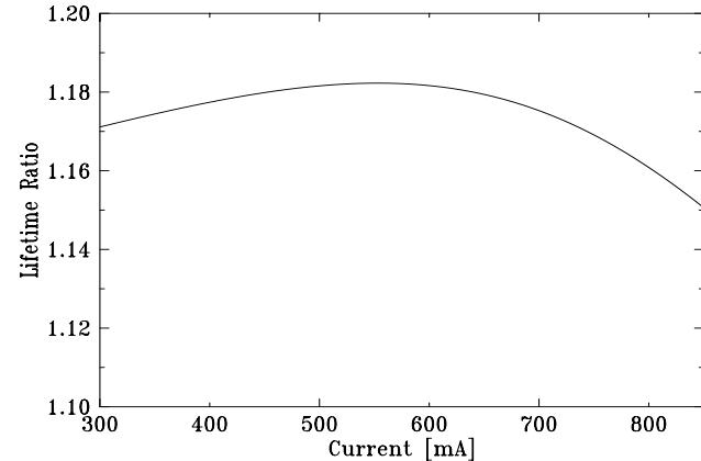
Figure 3: The measured increase in beam lifetime versus current after the periodicity restoration relative to before restoration.
