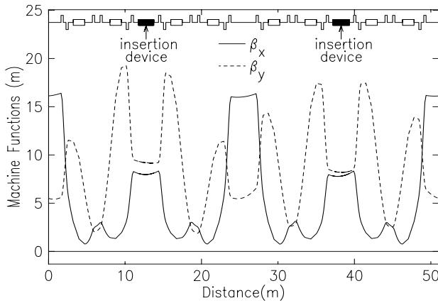
Figure 1: The  $\beta$ -functions in the NSLS VUV Ring calculated by LOCO as described in Section 2, before the periodicity restoration described in Section 3 was applied.
