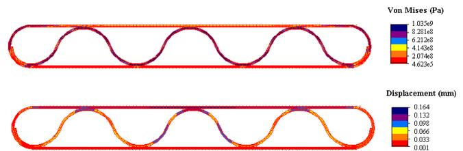
Figure 3. Laminar spring under 15 MPa load: stress and strain distributions.
