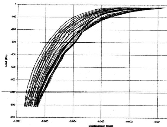
Figure 4. Laminar spring stress/strain: 10,000 cycles.
