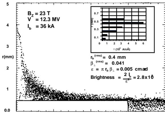
Figure 2. High-resolution diode simulation calculating the beam parameters.
