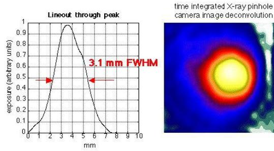
Figure 3a. Time-integrated x-ray images of the beam for  $B_z = 6$  T.
