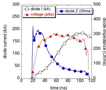
Figure 4b. The impedance of the HERMES-III diode decays with time, probably due to poor accelerator vacuum and oil contamination.
