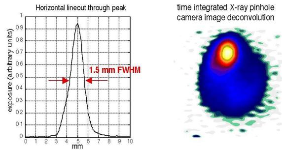
Figure 3b. Time-integrated x-ray images of the beam for  $B_z = 29$  T.
