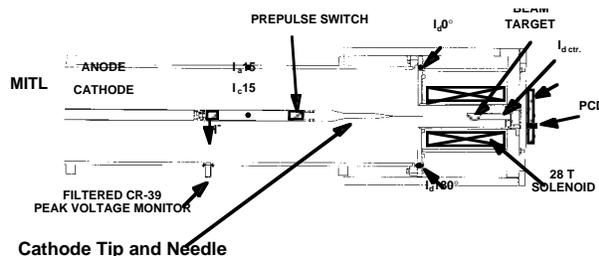
Figure 1. Schematic diagram of diode design and transition region, showing details and B-dot monitors.
