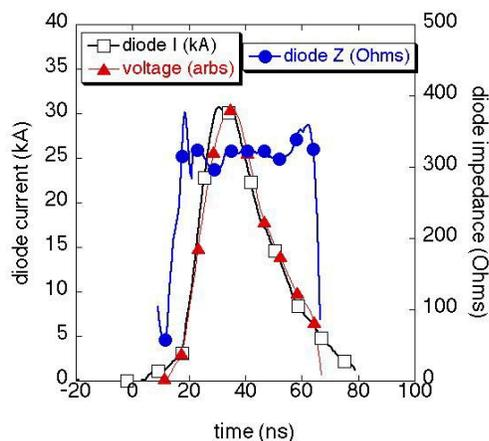
Figure 4a. A constant impedance diode shot with SABRE.
