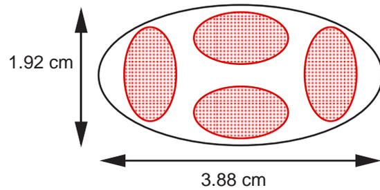
Figure: 3 Four beams emerging from the combiner.
