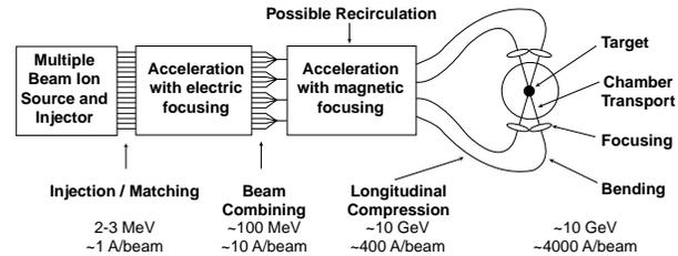
Figure: 1 Block diagram of an HIF induction linac driver.
