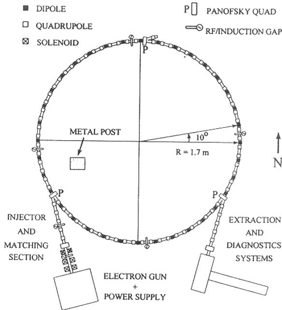
Figure: 11 Layout out of proposed electron ring at the University of Maryland.
