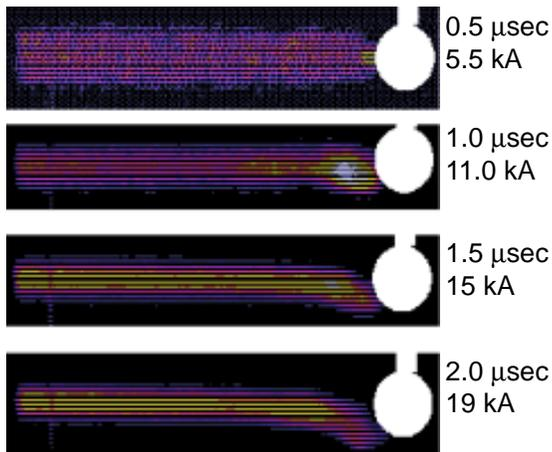
Figure: 6 Photographs of the plasma channel at various times after the laser trigger.
