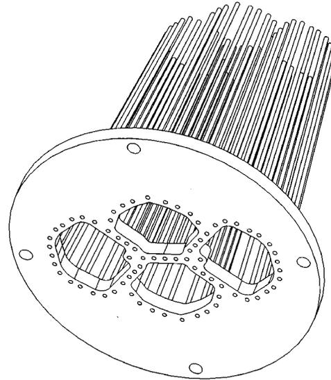
Figure: 4 The wire cage used for combining beams.
