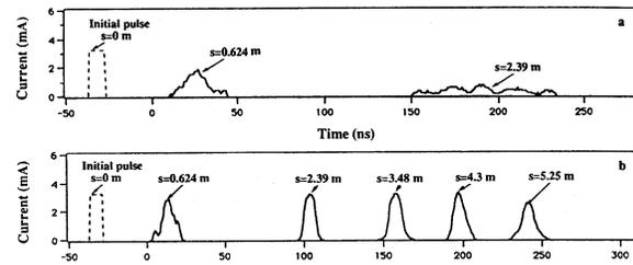
Figure: 10 Comparison between drift expansion and rectangular pulse restoration: (a) free expansion of a 300 eV, 3.3 mA, 7 ns bunch; (b) beam profiles with restoration.
