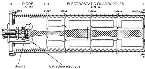
Figure: 2 Schematic Diagram of the 2-MeV ILSE injector.
