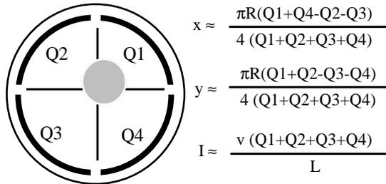
Figure: 8 The capacitive probe as non-interceptive beam diagnostic (R is radius, I is beam current, v is beam velocity, and L is probe length).
