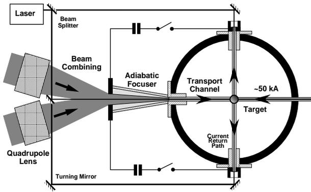
Figure: 5 A proposed scheme for final focus using adiabatic lenses and a discharge channel transport.
