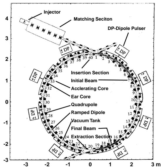
Figure: 7 Schematic diagram of the small recirculator.
