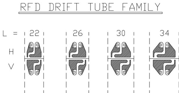
Figure 1: Cross Sections of RFD Drift Tubes.
