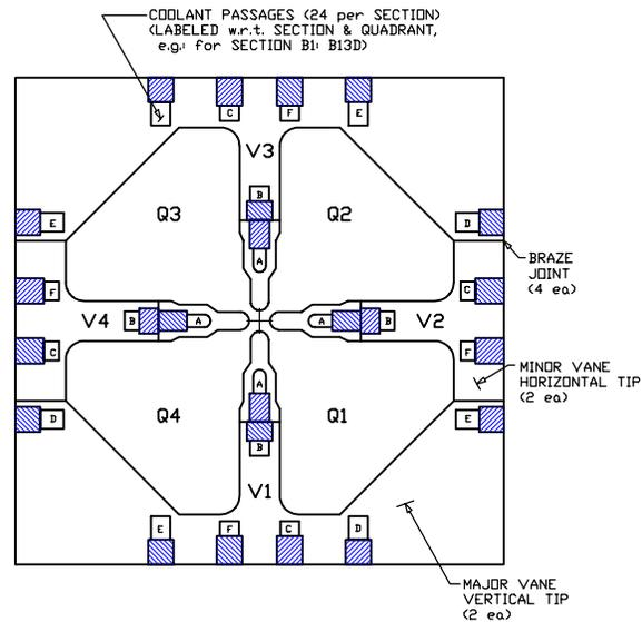
Figure 3: RFQ Cross-Section
