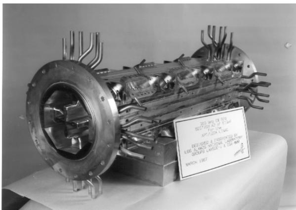
Figure 5: APT/LEDA RFQ Section A2 After Furnace Brazing
