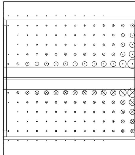
Figure 6: MAFIA plot of the magnetic field in a longitudinal section in the middle of the vertical plane.
