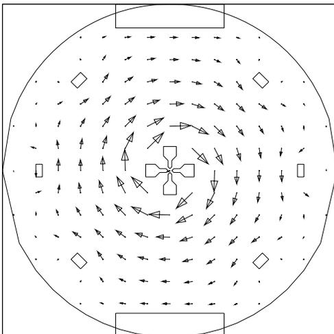
Figure 5: MAFIA plot of the magnetic field in a transverse section in the middle of the cell.
