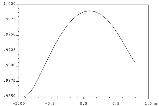
Figure 7: MAFIA plot of the normalized inter-electrode voltage.
