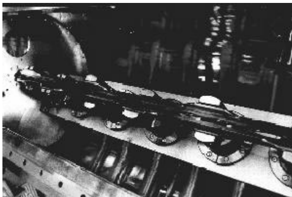
Figure 6: Electrodes mounted in the chamber.
