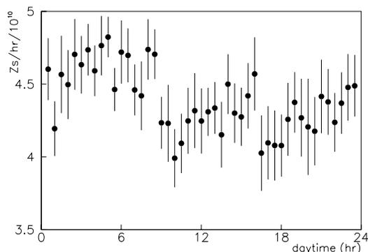
Figure 1: The diurnal luminosity during the 1996 SLC run. Shown is the luminosity normalized to  $10^{10}$  particles per bunch. The actual luminosity would be  $\sim 12$  times higher. A rate of 1 Z/hr is equal to about  $10^{28} \text{ cm}^{-2} \text{ s}^{-1}$ .
