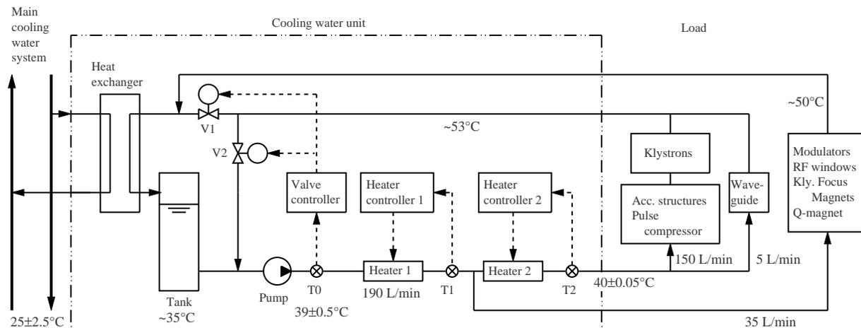
Fig. 1 Blockdiagram of the cooling unit.
