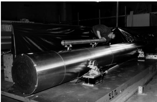
Figure 2: Regular girder for the 6m section including micro movers (short piece of structure on top to demonstrate the full assembly)
