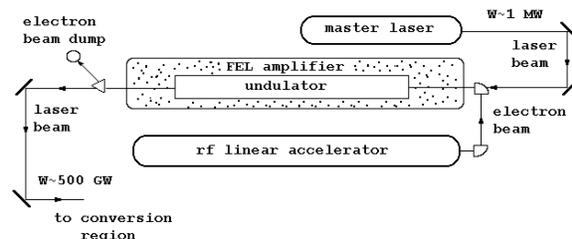
Figure 1: MOPA FEL configuration for a gamma-gamma collider
