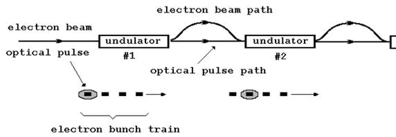
Figure 4: The scheme of multi-stage FEL amplifier. One optical pulse is amplified by a sequence of electron bunches. The peak power of the output radiation exceeds by a factor of  $N$  (number of amplification stages) the peak output radiation power of traditional single pass FEL amplifier.
