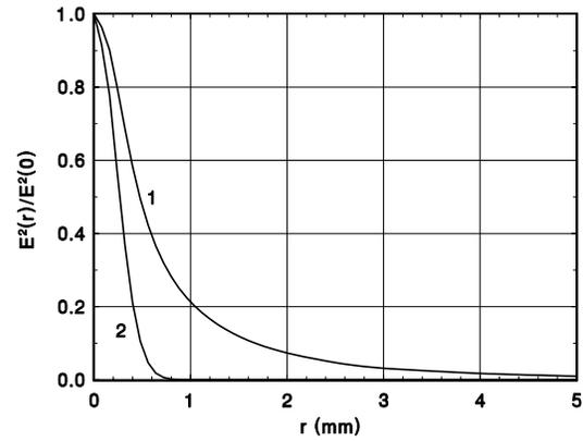
Figure 3: Radial distribution of the radiation power density (1) at the undulator exit and the electron beam current density (2).
