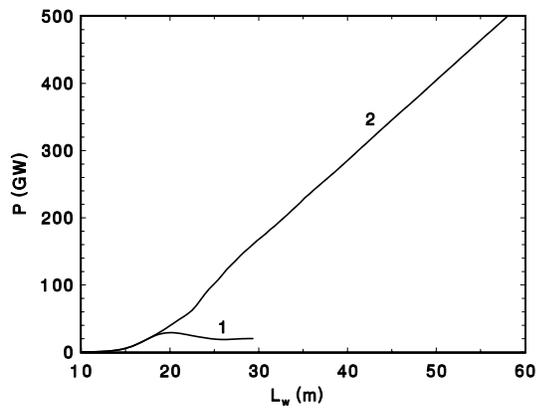
Figure 2: Output power of the FEL amplifier versus undulator length (curve 2). Curve 1 corresponds to untapered undulator.
