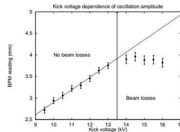
Figure 2: BPM coordinate reading as a function of the kick voltage.
