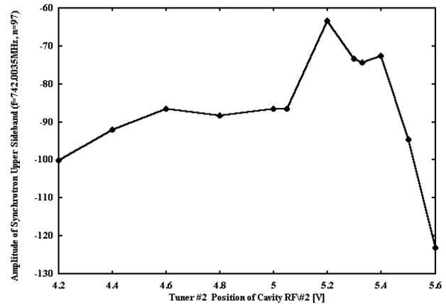
Figure 3: Oscillation amplitude (in dB) of the synchrotron upper dipole mode of  $n = 97$  (742.0035 MHz) as a function of the second tuner position of cavity RF #1.
