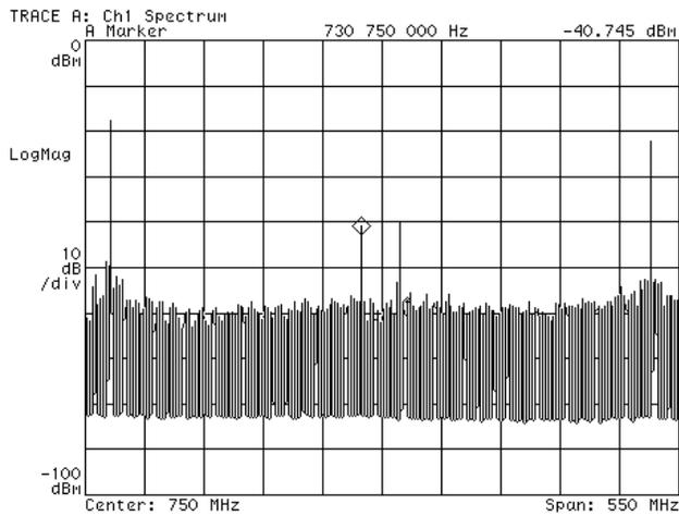
Figure 2: Beam spectrum for a quasi-uniform filling pattern. The second tuner is adjusted to an optimal position such that the spectral intensity fluctuations to be minimal.
