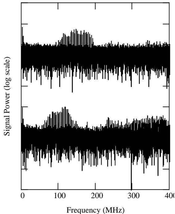
Fig. 2. The signal power at half intensity peaks at lower frequency. The intensity of the upper spectrum is twice that of the lower spectrum. The beam conditions are the same except for the beam intensity and the buncher voltage.
