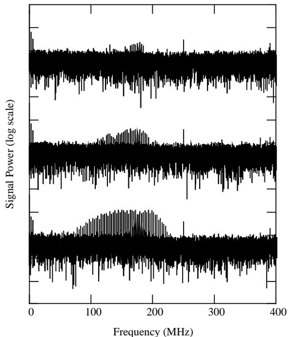
Fig. 1. Sideband power growing in time. The middle spectrum is 60  $\mu$ s after the top spectrum, and the bottom is 160  $\mu$ s after the top. All three spectra are from a single beam pulse.
