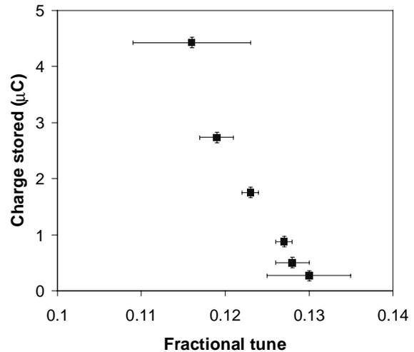
Fig. 4. Tune shift as a function of beam intensity.
