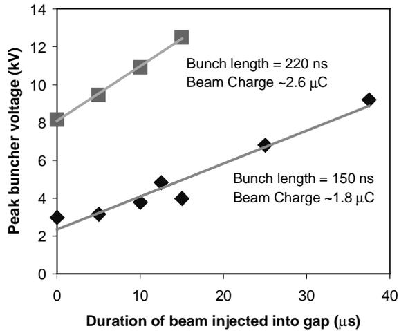
Fig. 3. The instability threshold is decreased (more buncher voltage is required) when beam is injected into the gap. The straight lines are linear fits to the data.
