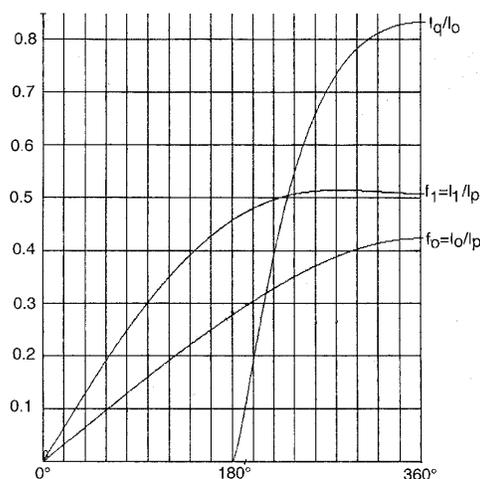
Figure 4. Tube current form factors calculated by W. Pirkel. Bottom axis is conduction angle of tube. All measurements were made with an angle of  $190^\circ$ - $200^\circ$ .
