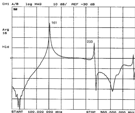
Figure 3. Anode impedance as a function of frequency with an electrical short across the output of the amplifier.
