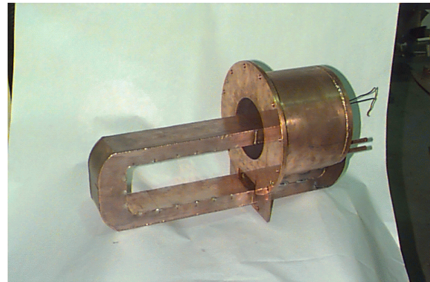
Figure 3: Ferrite tuner for the 9.77-MHz fundamental frequency cavity.
