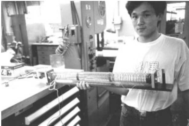
Figure: 4 Fenghua Liu holding the 70 cm long ZMEVVA during assembly and coil winding.
