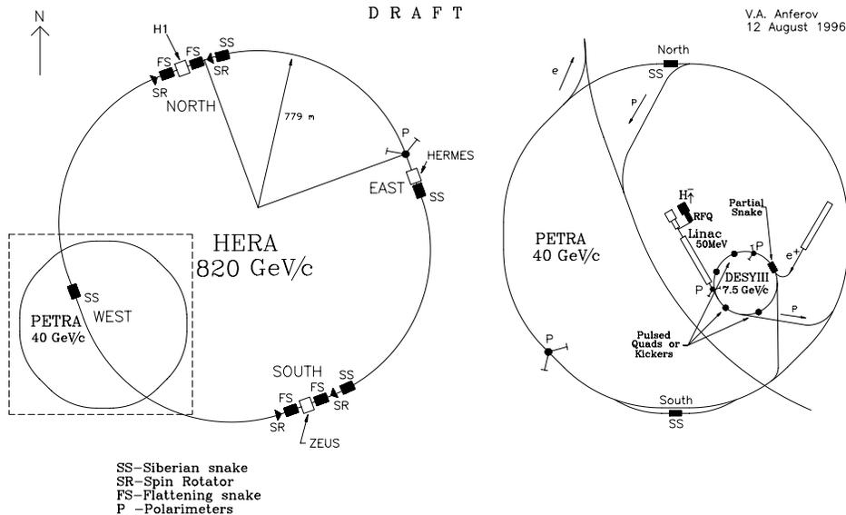
Figure 1: The proposed modifications for an 820 GeV/c polarized proton beam at DESY.
