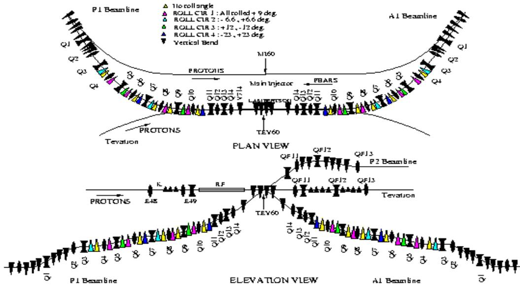
Figure 1. Plan and elevation of the P1, A1, and P2 beamlines in relation to the Main Injector and the Tevatron. The drawing is not to scale. The Main Injector and Tevatron magnets are not shown on the plan view for clarity.
