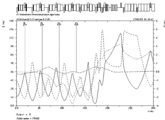
Figure 4. Lattice functions for the P1 beamline match into the Tevatron.
