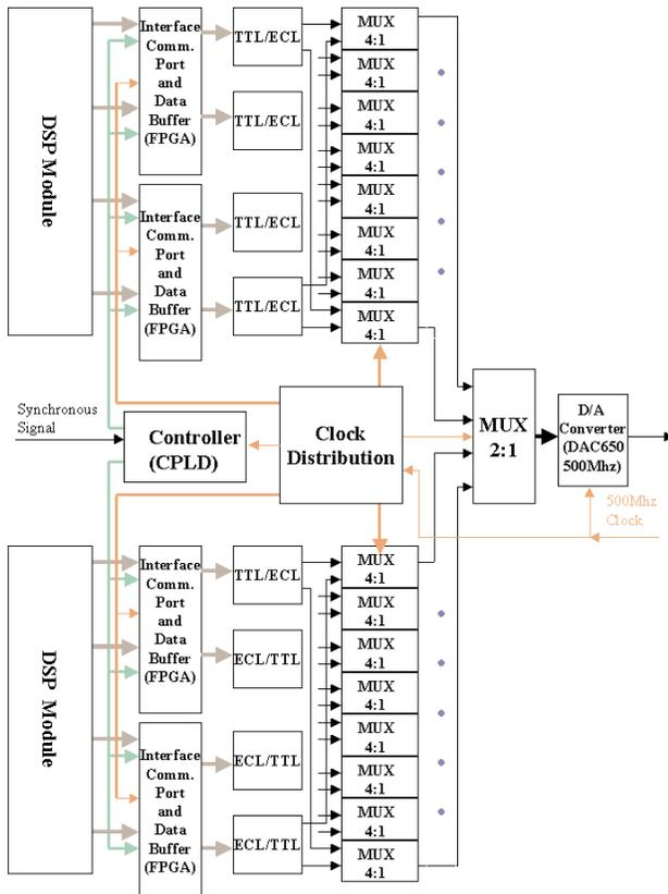
Figure 2: Functional Block Diagram of the DAC/MUX Unit
