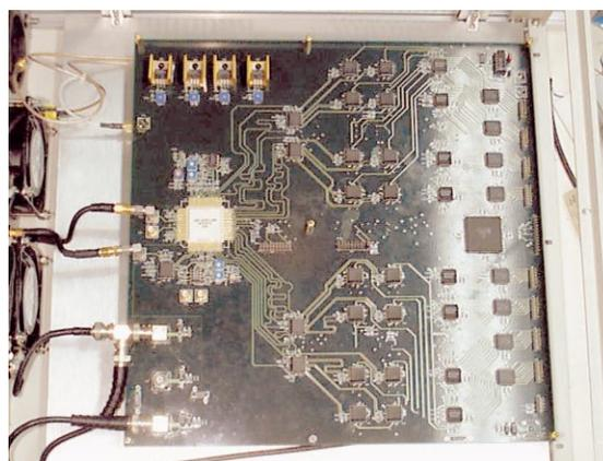
Figure 1: The ADC/DEMUX unit has been built and tested successfully
