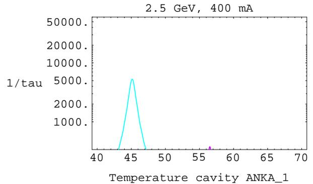
Fig. 5: Transv. vertical growth rates vs. temperature
