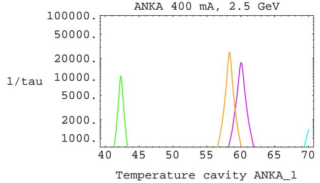
Fig. 3: Longitudinal CB growth rates vs. temperature
