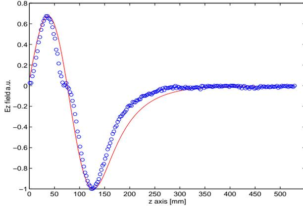
Figure 2: Measured electric field on half cavity length for the L9 mode (dotted line), compared with the computed field (solid line).
