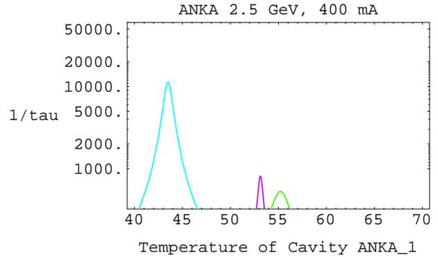
Fig. 4: Transv. horizontal growth rates vs. temperature
