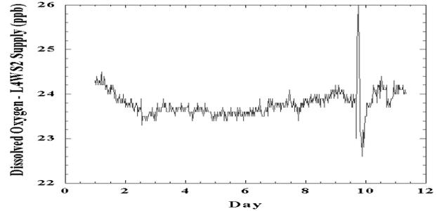
Figure 3: Dissolved oxygen [ppb] over an 11-day period in one LCL with oxygen-scavenging resin.
