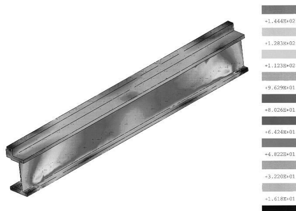
Figure 1: Girder distortion energy (color fringe plot)
