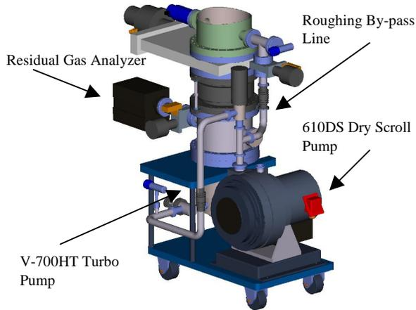
Figure 2: Details of the Insulating Vacuum System Station
