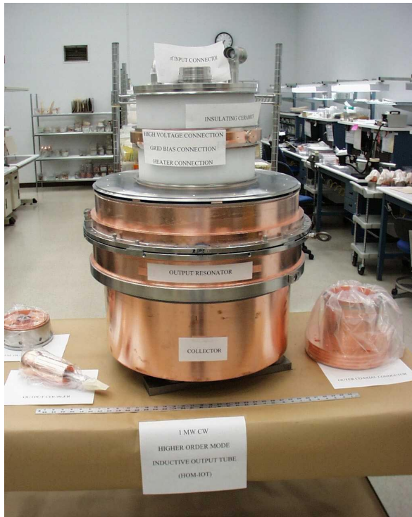
Figure 5: 1 MW CW HOM-IOT (prototype)
