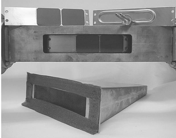
Figure 2. HOM load individual panel test setup.
