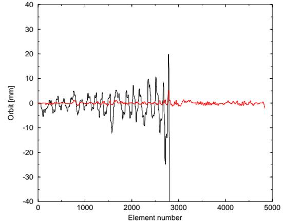
Figure 5: Simulated first turn orbit correction in RHIC, vertical plane.
