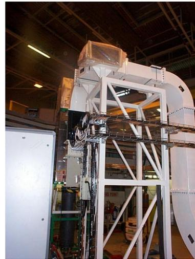
Figure 3. Klystron with Waveguide Switch in Position.
