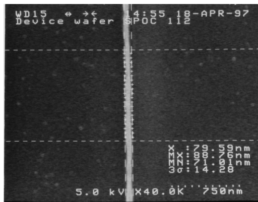
Figure 5. Scanning electron micrograph of 80 nm isolated line gate structure in DUV resist.
