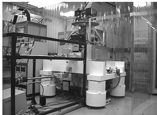
Figure 4 Photograph of SCALPEL exposure system at Bell Labs. It takes up roughly the same amount of space as an optical lithography tool.
