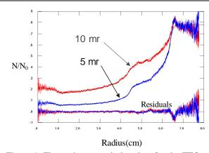
Figure 1, Fits to the transmission data for the FTO. The upper two curves are the measured transmission vs. radius. The bottom curves are the residuals of the two fits.
