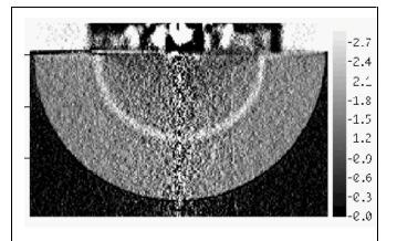
Figure 2. Reconstructed density of an exploding onion skin 1.9  $\mu$ s time after detonation. The scale on the right is grams per cm<sup>3</sup>.
