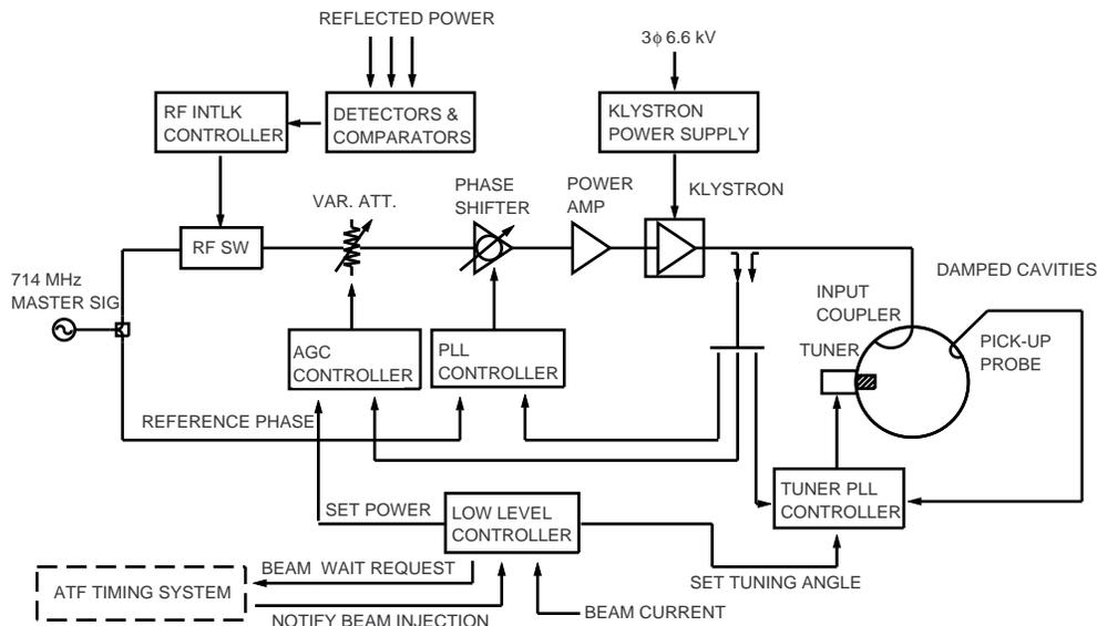
Fig. 3. Conceptual block diagram of the low-level system.
