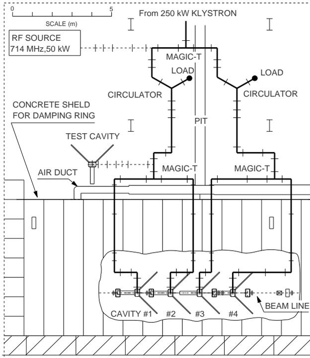
Fig. 2. Layout of the RF system. Top view.
