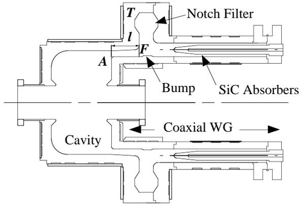
Figure 1: A schematic drawing of the test cavity
