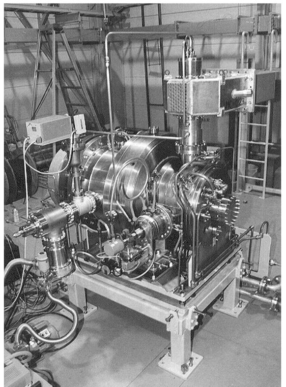
Figure 2: The test cavity with an input coupler and a tuner installed.
