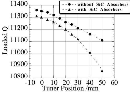
Figure 3: The loaded-Q responses to the tuner position for the cavity with/without the absorbers.
