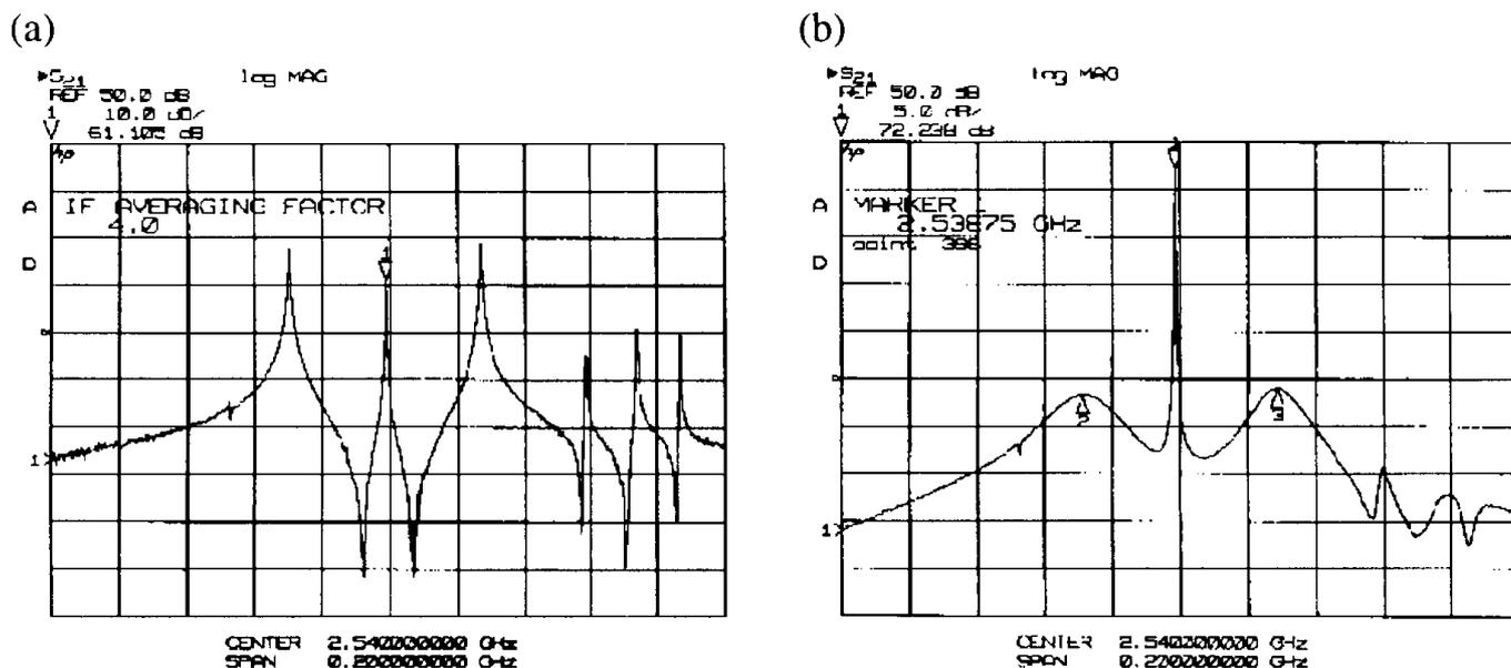
Figure 5: Measured transmission between beam ports at a-cavity: (a) coupling cavity is not damped and (b) is damped.
