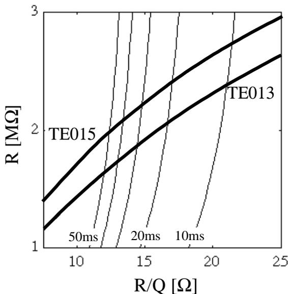
Figure 6: Chart used for comparison between the TE013 and TE015 s-cavity.
