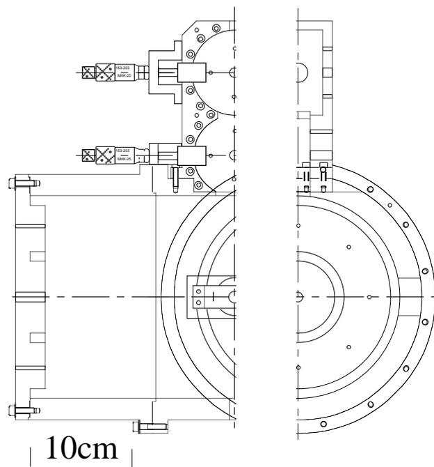
Figure 1: First cold model of ARES without a damper at the c-cavity.
