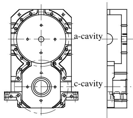
Figure 4: Modified c-cavity for coaxial couplers.
