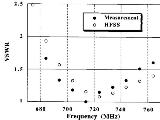
Figure 1: VSWR of the cold model of ATF input coupler.
