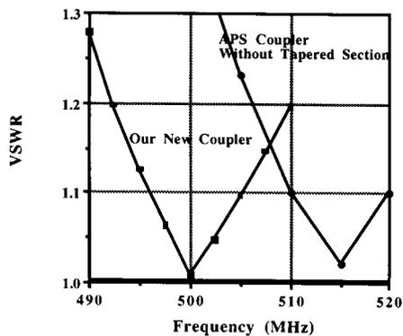
Figure 8: VSWR of our new coupler and that of APS coupler without its tapered section.
