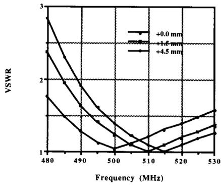
Figure 6: VSWR versus the position of short plate of coaxial line.
