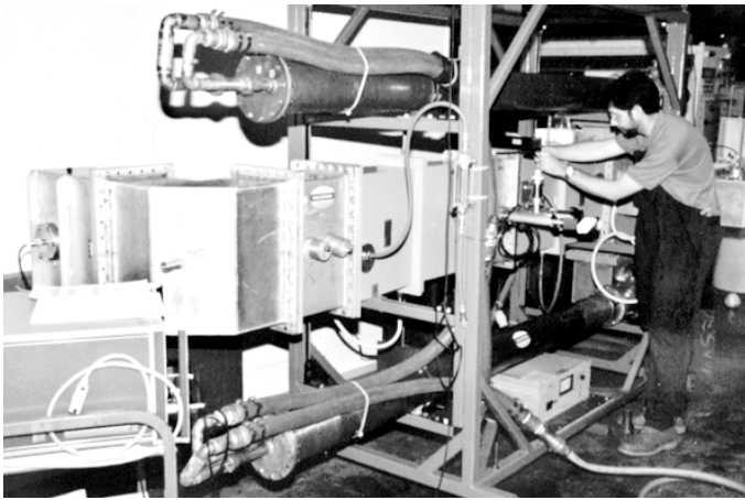
Fig. 8: Typical high power processing set up showing two windows and two 300 kW water loads.
