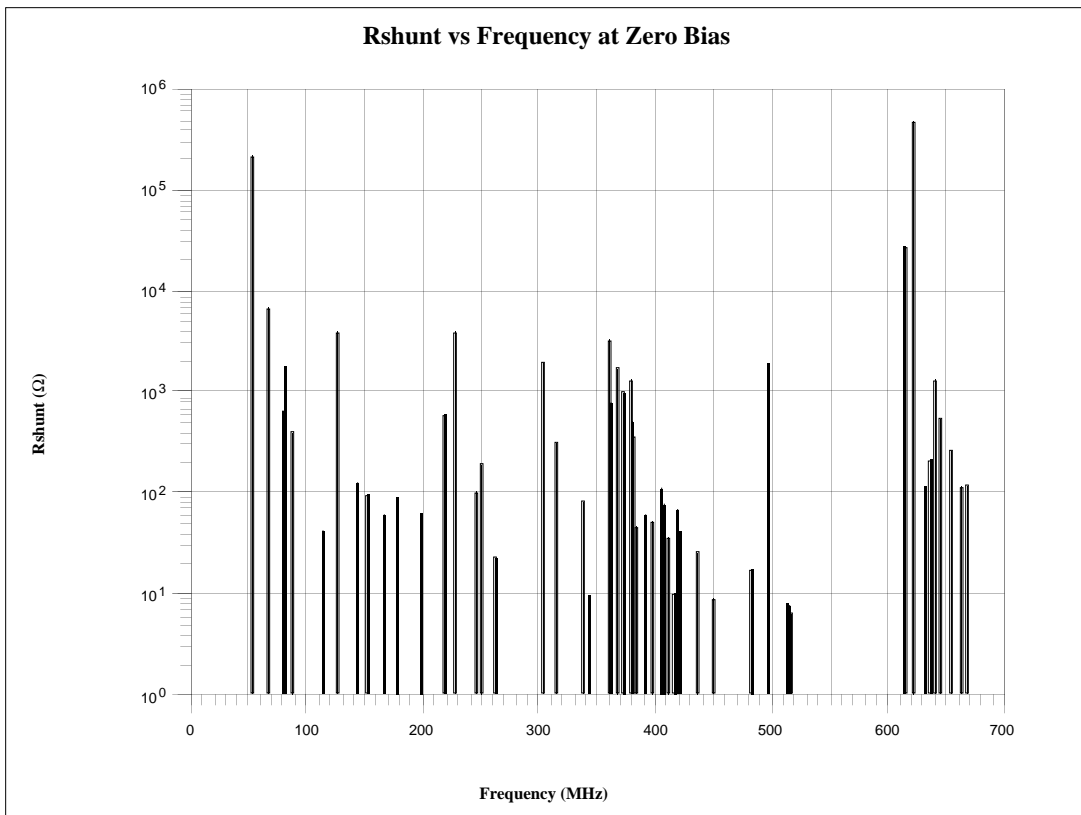
Figure 4: Shunt Impedance at Zero Bias of Main Ring Cavity.
