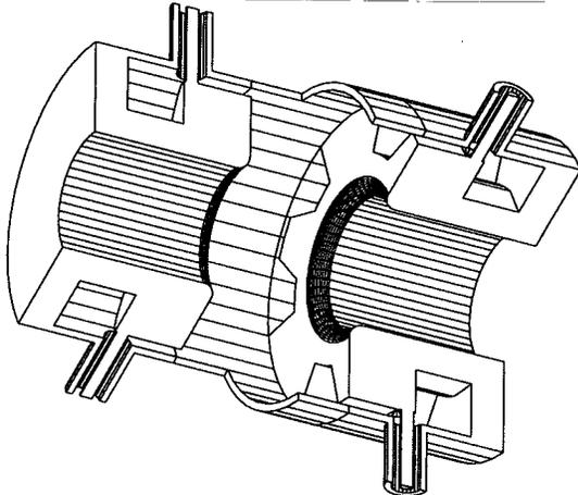
Figure 6: CAD view of the overdamped kicker cavity.
