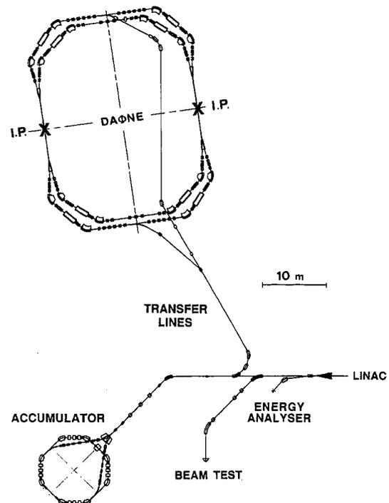
Figure 1: Layout of DAΦNE and its injector.
