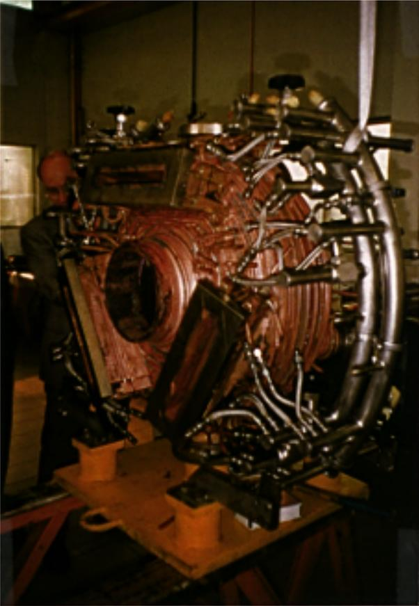
Figure 4: DAΦNE RF Cavity during fabrication at Zanon.
